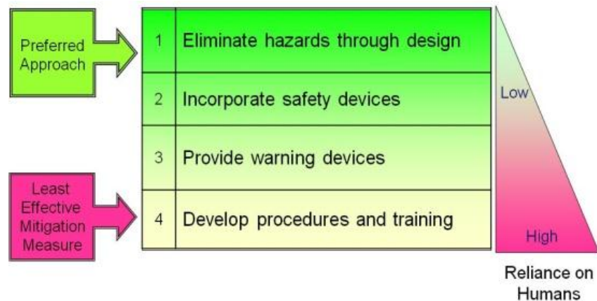
Figure 2 — System Safety Order of Precedence
